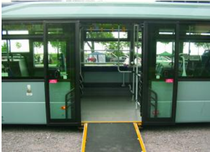
Low floor bus with extended ramp.
